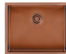
Volta Single bowl Ref. VL500DBC £485 Overall size: 540/440 mm Bowl size: 500/400/190 mm Cutout size: 520/420 mm (Inset) Minimum cabinet size: 600 mm Waste included: 90 mm BSW
